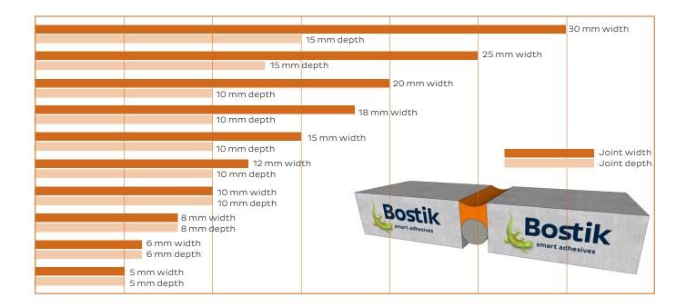
To apply the sealant with the correct depth, a backer rod is used. Backer rods are used to control the depth of sealant, to provide backing for the sealant during application and to prevent triple bonding. Materials used as backer rods should be weaker than the sealant itself and not obstruct the movement capability of the sealant, whilst compressing or expanding.
